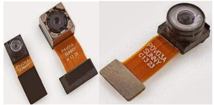
Fig.2 Front and Rear Camera Fig.3 Fish-eye lens
