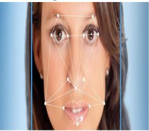
A facial recognition system analyses the shape and position of different parts of the face to determine a match. Surface features, such as the skin, are also sometimes taken into account.
