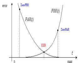
False acceptance rate (FAR) and false rejection rate (FRR) as functions of the threshold t
